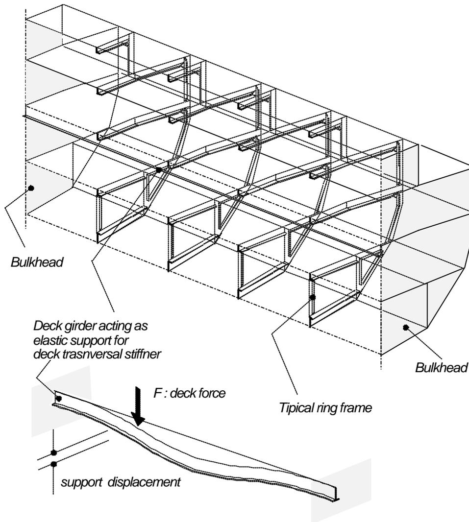
Figure 1 – Elastic constant support for the frames
